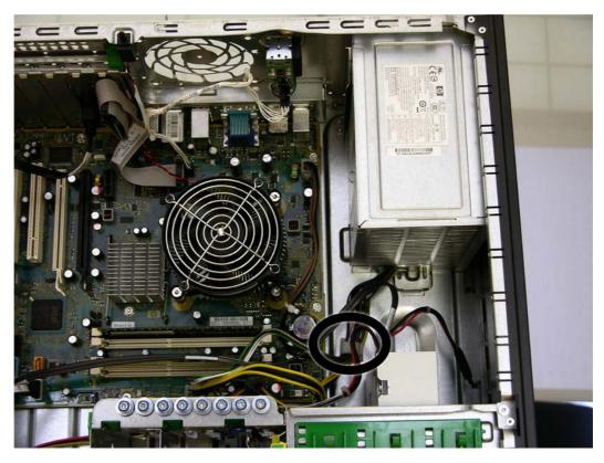
5. Remove the two Torx screws (1) and the two security screws (2) that connect the power supply to the chassis.
